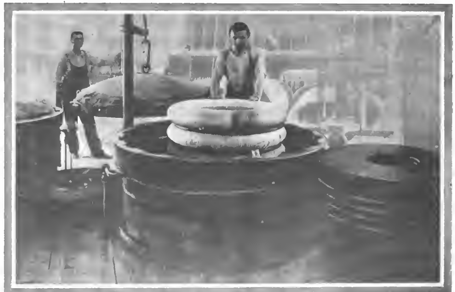
Curing tires at the plant of the Federal Rubber Mfg. Co., Milwaukee, Wis.
